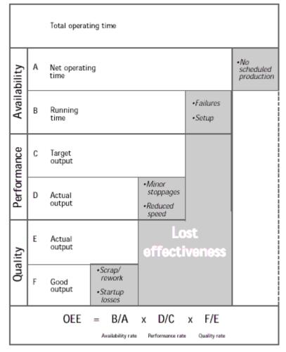
Bars E and F show quality. As you can see, the actual output (E) is reduced by defect losses such as scrap and startup losses, shown as the shaded portion of bar F.
